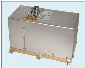
Rubidium atomic frequency standard clock, Source:ESA
